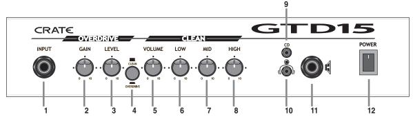
**1. INPUT:** Use this jack to connect your guitar to the amplifier by means of a shield-ed instrument cable.
